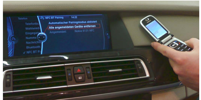
Figure 5: NFC-based Bluetooth Pairing in the car.
